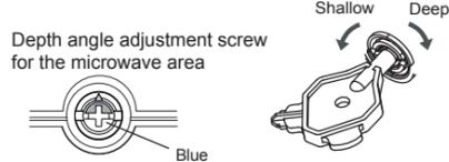
Use the area adjustment tool (B) as shown above to change the area depth angle.
